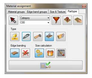
When BOM is generated, the parts are accounted for according to their type. The parts of the same type are grouped together. The size of each part is calculated as well as the amount of materials necessary for manufacturing. All materials are sorted by material type, thickness, etc.
