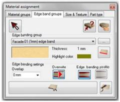
One can change the thickness of edge banding for the entire group. For example, the designer decides to use 2mm edge banding instead of 1mm. He/she can use the filter to select the edge banding that meets the search criteria and reassign it. Banded edges may be highlighted. One can also select the edges that are invisible from that angle without rotating the furniture model.
